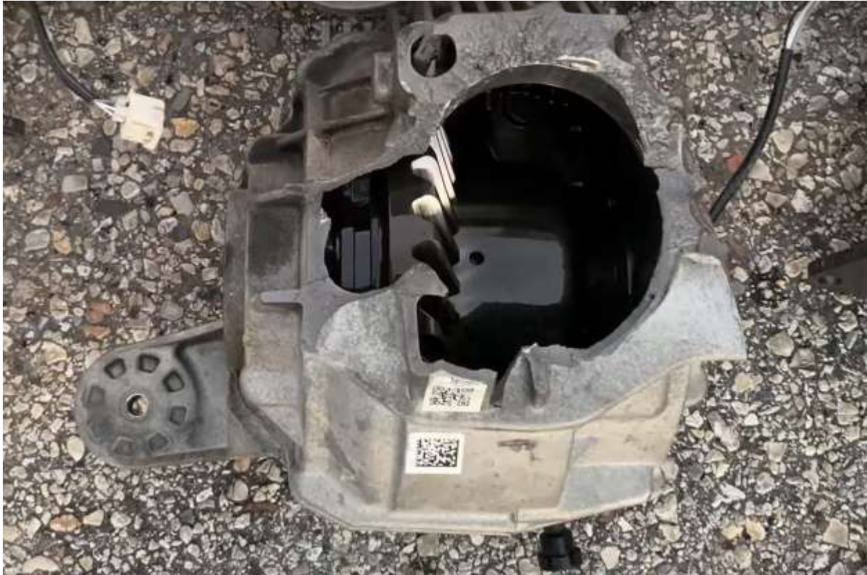
© YouTube | Olson's Ecoboost | The no-longer-intact rear differential from the stock Demon in the video. Note the missing front half and pinion gear.
