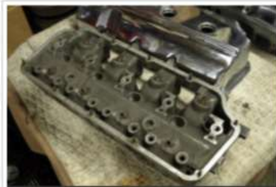
Part of Chrysler's strategy for the upcoming 1965 race season was to drop as much weight from the cars as possible – particularly at the nose. While the 1965 Race Hemi cylinder heads were essentially identical to their 1964 counterparts from a design and performance standpoint, they differed in that aluminum had replaced cast iron as the material of choice. The weight of each head dropped from 60 to 27 pounds from that change alone, resulting in a 66 pound weight reduction at the front of the car overall. Image: FCA
