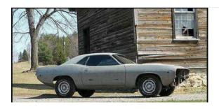
This Tooling Proof Body was the first assembled steel body for the 1974 model year. It was used as a gauge to take measurements from checking the alignment of body panels for production cars.
